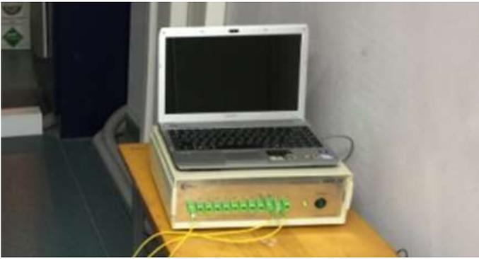
**Picture 1.** The control unit of fiber-optic system for temperature measurement
